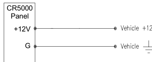
FIGURE 1.6-2. Alternate Connect on to Vehicle Power Supply
