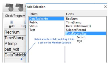
LoggerNet users, select **Main** and click the **Connect** button ( on the LoggerNet toolbar, select the datalogger from the **Stations** list, then click the **Connect** button ( once connected, you can select a table to view using the **Table Monitor** list.
