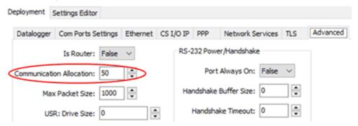
• USR drive: Optionally allocated. Holds image files. Holds a copy of final-storage memory when TableFile() instruction used. Provides memory for FileRead() and FileWrite() operations. Managed in File Control. Status reported in Status table fields USRDriveSize and USRDriveFree.
