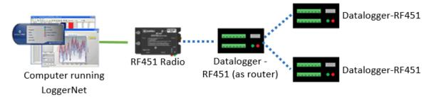
To configure an RF451 radio to communicate with multiple dataloggers, you must complete the following steps (instruction follows):
