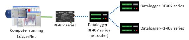
To configure an RF407-series radio to communicate with multiple dataloggers through a router, you must complete the following steps (instruction follows):
