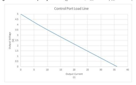
o 3.3 V Logic Level Drive Capacity: 10 mA @ 1.8 Vdc;  $V_{out} = 3.3 \text{ V} - (I_{out} \times 150 \Omega)$
