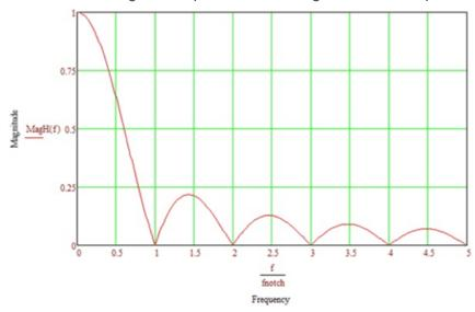
Filtering comes at the expense of measurement time. The time required for filtering is equal to  $1/f_{N1}$ . For example, setting  $f_{N1}$  equal to 50 will require 1/50 sec (20 ms) for filtering. As  $f_{N1}$  is set to smaller values, random noise in the measurement results decreases, while measurement time increases. The total time required for a single result includes settling + filtering + overhead.
