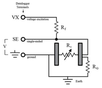
With  $R_g$  in the resistor network, the signal measured from the sensor is described by the following equation:
