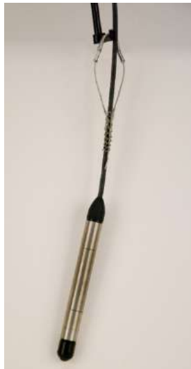
FIGURE 7-1. Transducer suspended with split mesh cable grip
