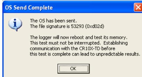
The information in the dialog helps to corroborate the signature of the operating system sent. For devices such as the CR10X (especially those with extended memory) that can take a long time to reset following an OS download, text warns you against interrupting the memory test.
