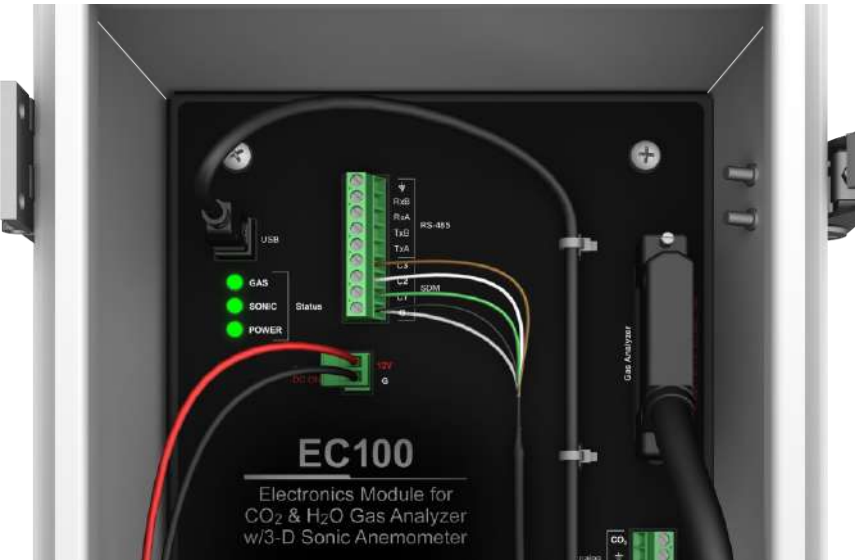
FIGURE 8-3. LED status during normal operation
