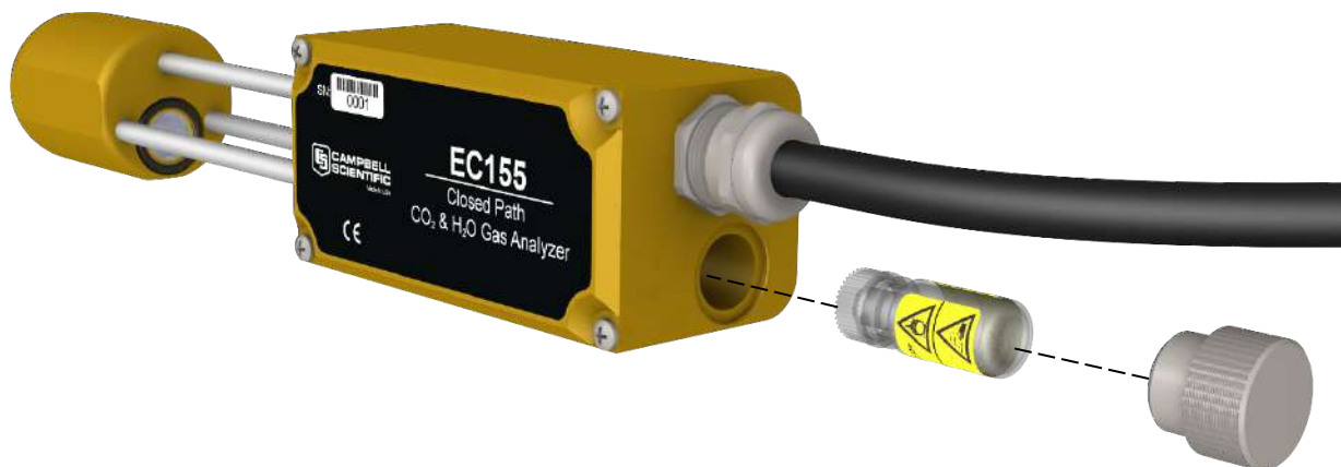
FIGURE 9-11. Replacing the source housing desiccant/scrubber bottle (replacement bottles purchased in or after July 2017 may appear different than in the figure)
