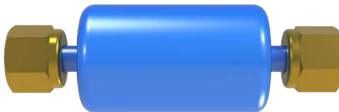
FIGURE 9-1. The vortex filter assembly (pn 32203) includes a 25 \mu m particulate filter with 1/4-in Swagelok® nuts on either side.
