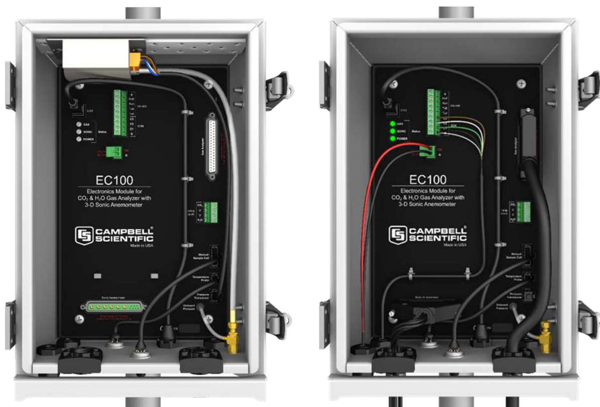
FIGURE 6-11. EC100 electronics front panel. The left figure shows the panel as it is shipped from the factory (enhanced barometer shown). The right figure shows the panel after the user has done all the wiring and made all connections (basic barometer used).
