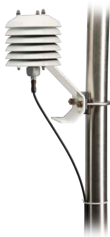
FIGURE 7-4. HMP60 and RAD06 Radiation Shield on a tripod mast
