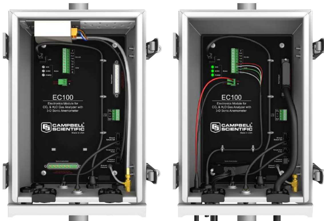
FIGURE 6-5. EC100 electronics front panel with enhanced barometer. At left, as received from Campbell Scientific. At right, all wiring and connections complete.
