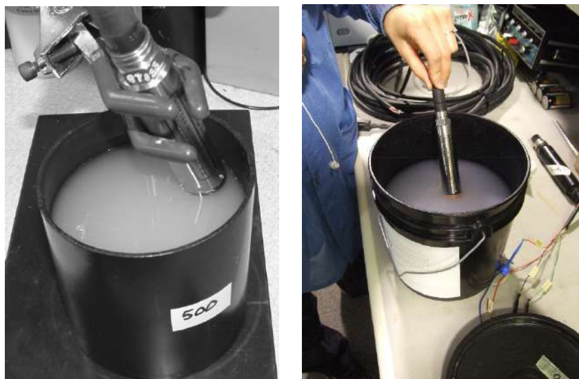
FIGURE 8-3. OBS-3+ (left) and OBS300 (right) in 500-NTU AMCO Clear® turbidity standard in 100-mm black polyethylene calibration cup
