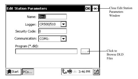
On this screen you can change the station **Name**, select the **Datalogger** model, enter any **Security Code**, select which Allegro CE **Communication** port you are using to connect to the datalogger, and associate a **Program**. When you are finished editing the station parameters, touch **OK**.
