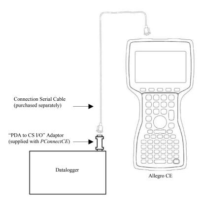
Note that one side of the connector is labeled Datalogger, and the other side is labeled PDA. If the connections are reversed, communication with the datalogger will fail.
