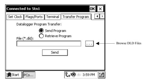
First, select the desired option, and then touch the Browse button to the right of the File field to choose the file to be sent or to enter a name for the retrieved file. After the File field is completed, press the Send (or Retrieve) button.
