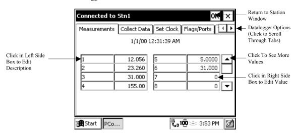
Because of the small screen size, you may see only a portion of the input locations in the datalogger. Touch the up or down arrows to the right of the measurement cells to scroll through the values.
