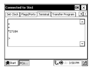
To return the datalogger to its program execution state, enter \*0. LOG1, LOG2, or LOG12 should be displayed indicating that the code in program table 1, and/or program table 2, is running.
