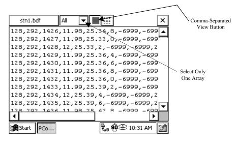
As you scroll through the data, note that all of the collected arrays are displayed intermixed as they were retrieved from the datalogger. To graph a column of data, you must limit the display to only one array type. Tap the Array ID dropdown arrow and select the ID of the array from which you want to graph data. Double tap the column of interest to graph it. You can scroll back and forth within the data. To see the value and the time stamp of a particular point, just tap that point.
