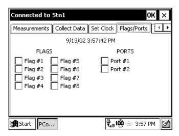
To change the state of a port or flag, touch the box for that port or flag. There may be a small time lag between when the box is touched and when the state of the port or flag appears to change.
