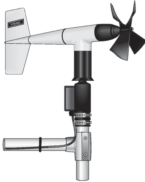
Figure 5-1. Wind Monitor Mounted to a CSC Crossarm
