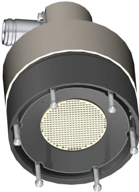
Figure 9 Remove 6 screws from the transducer housing
