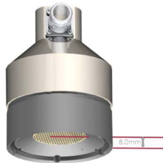
Figure 4 Distance from edge of transducer housing to grill
