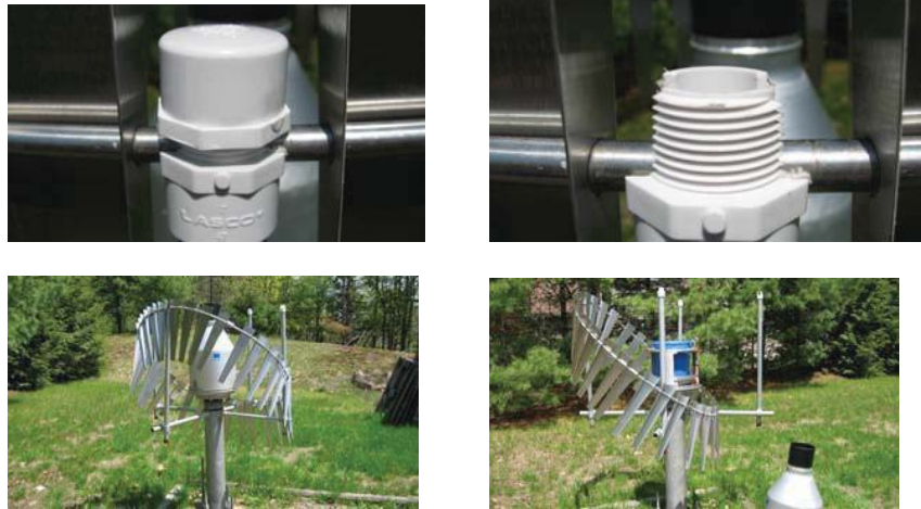
FIGURE 8—1. Removing the Alter wind screen from 3 of 4 posts
