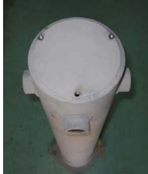
FIGURE 6—5. Orientation of mounting holes on pedestal
