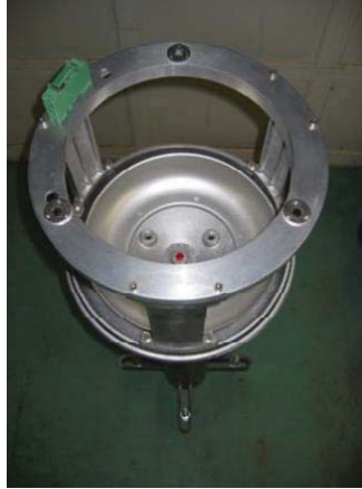
FIGURE 6—7. Sensor frame on pedestal with proper orientation
