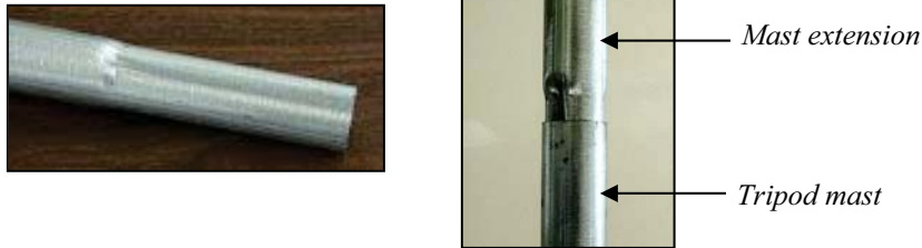
Figure 4: Drive the tapered end of the mast extension (left) into the tripod mast. If using two extensions, drive the tapered end of the second extension into the top of the first extension.
