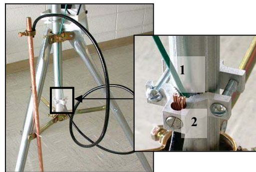
Figure 18: The TP1-GK assembly. Right is the 14 AWG wire and the #4 cable attached to the tripod coupling.
