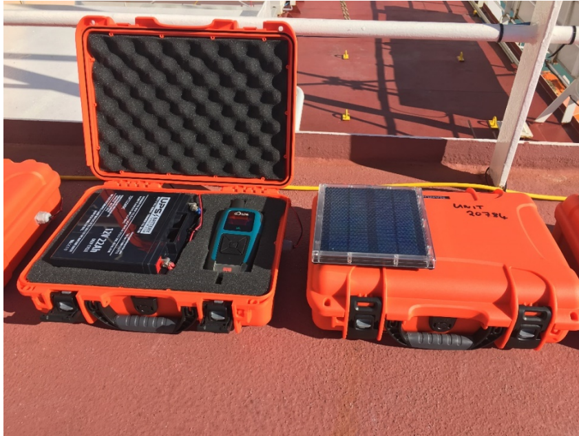
Figure 3: Iceberg tracking beacons built by Abby Dalton and Luke Copland. Three of these beacons were deployed onto icebergs in Baffin Bay and four were deployed onto icebergs within Trinity Fiord to monitor their movement. GPS trackers transmit their position using the Iridium satellite network and can be programmed remotely to modify transmission frequency according to activity (e.g. less frequent transmissions during winter when they are frozen in sea ice and have minimal movement). Photo: Luke Copland.
