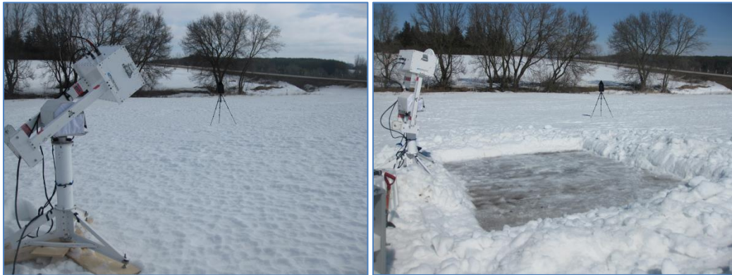
Figure 3 Scatterometer configuration shown. At left, natural snow cover is being scanned. At right the excavated area can be seen.
