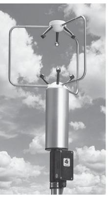
may be selected. Each 81000 is individually wind-tunnel tested and calibrated to compensate for wind shadow effects of the support structure.
