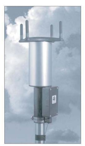
for wind speed and wind direction. A variety of serial output formats are also available on the standard sensor. These include ASCII text, RMYT (compatible with YOUNG displays), NMEA and SDI-12 formats.
