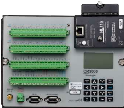
The NL116 Ethernet/CompactFlash module is shown attached to the CR3000's peripheral port.
