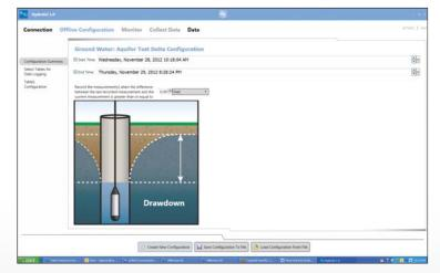
HydroSci software simplifies the process of configuring the sensor to monitor surface water, ground water, or a standard pump test (shown above).
