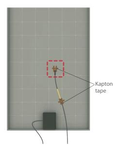
Kapton tape is required for cable strain relief. The tape is also used to fasten the CS240 to the back of a solar panel when the temperature may exceed 70°C.
