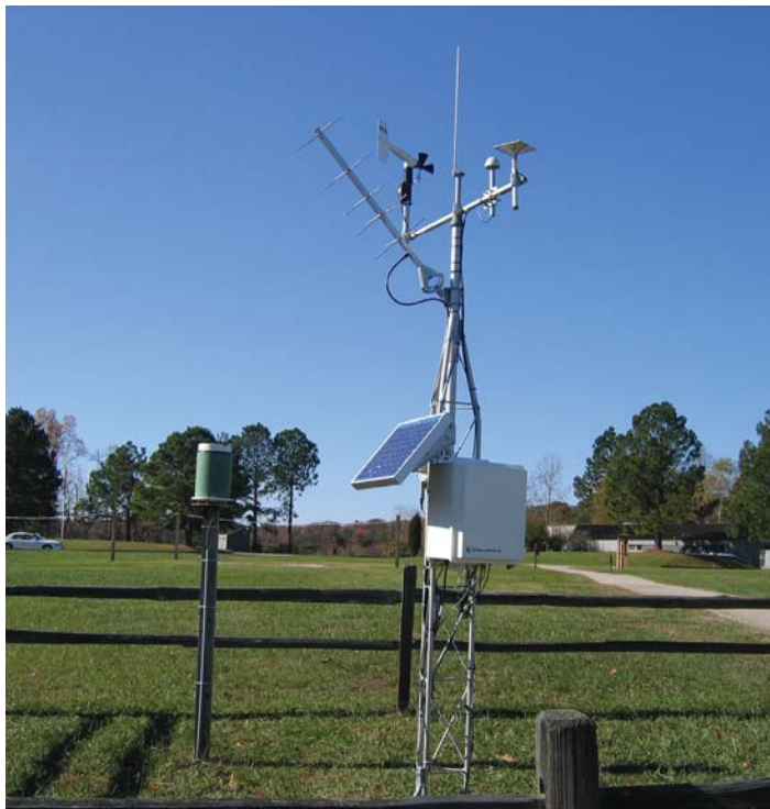
This station for the National Estuarine Research Reserve (NERR) in Virginia transmits data via our GOES satellite transmitter.
