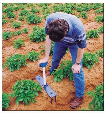
Specialized tools and techniques offered by Campbell Scientific simplify probe installation while minimizing soil disturbance.
