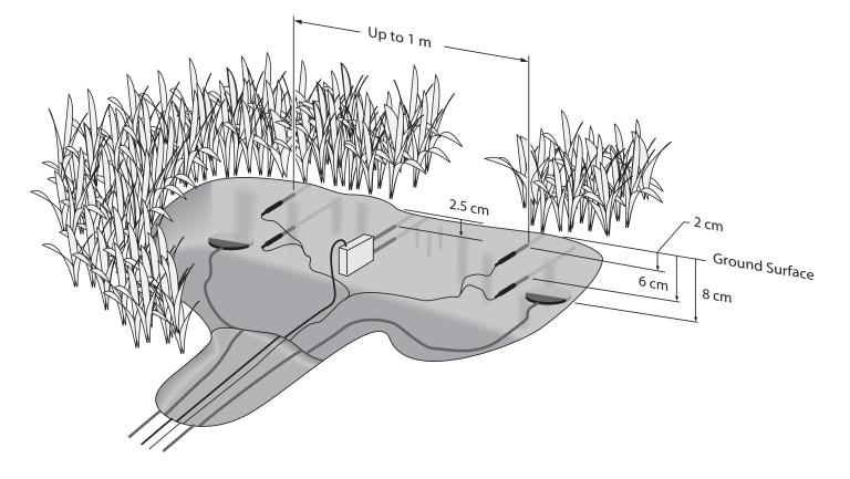
Above is an example energy-balance installation. The HFP01SC Heat Flux Plates are installed with the CS616 Water Content Reflectometer and TCAV Averaging Soil Temperature Probes. All sensors must be completely inserted into the soil face before the hole is backfilled.
