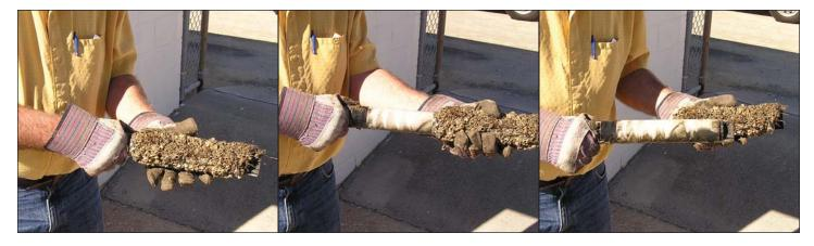
The OBS500 has a plastic sleeve option that can simplify cleanup. The three above photographs show the sleeve being removed.
