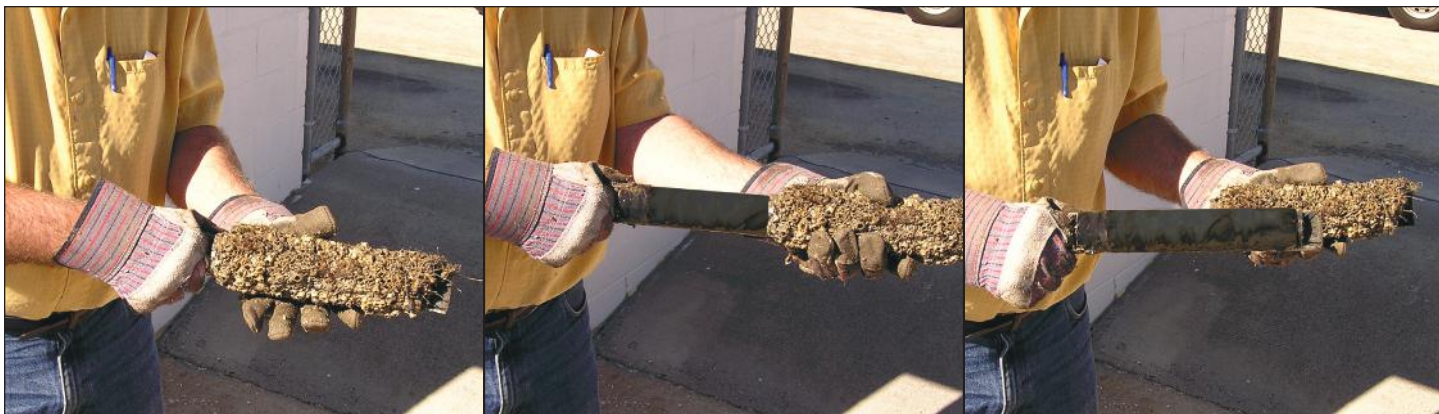
Two sleeve options are offered by Campbell Scientific. The three above photographs show the plastic sleeve being removed.
