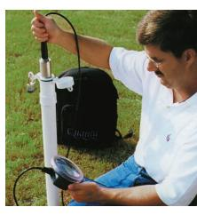
comprises the Quanta•G transmitter, a cable (up to 100 meters) and a Quanta display. Utilizing state-of-the-art technology and modern manufacturing principles, Hydrolab is able to offer the Quanta•G at a fraction of the price of other multi-parameter instruments, without compromising data quality.
