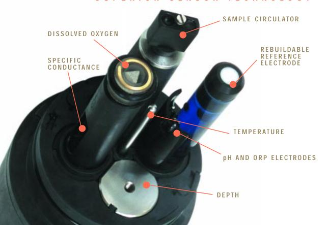
pH – Hydrolab uses a standard pH glass sensor and unique rebuildable reference electrode.
