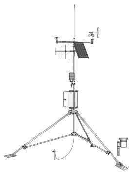
Field stations are located at the measurement site. The above field station uses a Yagi antenna to transmit the data.
