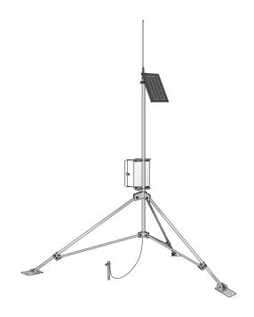
Repeater stations act as communication relays between stations that cannot communicate directly due to distance or obstacles. Repeater stations use omnidirectional antennas.
