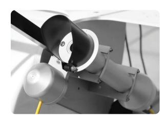
**SHP1** Pyrheliometer is a combination of the CHP 1 design and sensor technology with our smart interface advantages that make the SHP1 the best commercially available pyrheliometer. Key features are digital signal processing and interfaces optimised for industrial data acquisition and control systems.
