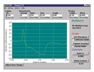
PCTDR displays waveforms for system setup and troubleshooting. A CD containing PCTDR is shipped with each TDR100 Reflectometer. This software is also available, at no charge, from our website.
