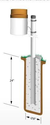
At left is a TE525 mounted onto a CM310 pole that is embedded directly in a concrete pad (-NP no pedestal base option).
