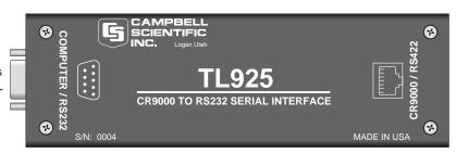
A standard 9-pin cable (CSI Model SC12 or SC12R or equivalent) is required between the PC and TL925. The SC12(R) is approximately 2 feet in length; a customer-supplied equivalent can be up to 50 feet. If the computer has a 25-pin serial port, a DB25 to DB9 adapter cable is required. For IBM PC or compatible computers, Campbell Scientific's PC9000 Support Software supports data retrieval, program upload/download, monitoring and real-time graphical display of data.
