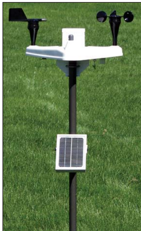
WeatherHawk provides real-time weather measurements and calculates ETo on an hourly and daily basis.
