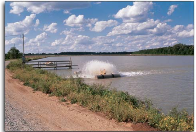
Aerators are activated only when dissolved oxygen is low.
