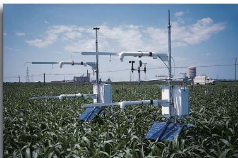
Bowen ratio systems measure temperature, water vapor, and carbon dioxide gradients over sorghum (Lincoln, NE).
