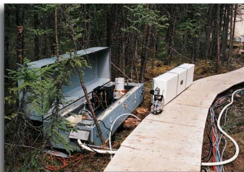
A trace gas analyzer uses TDLAS technology to measure N_2O or CH_4 fluxes during BOREAS (Prince Albert, SK, Canada).
