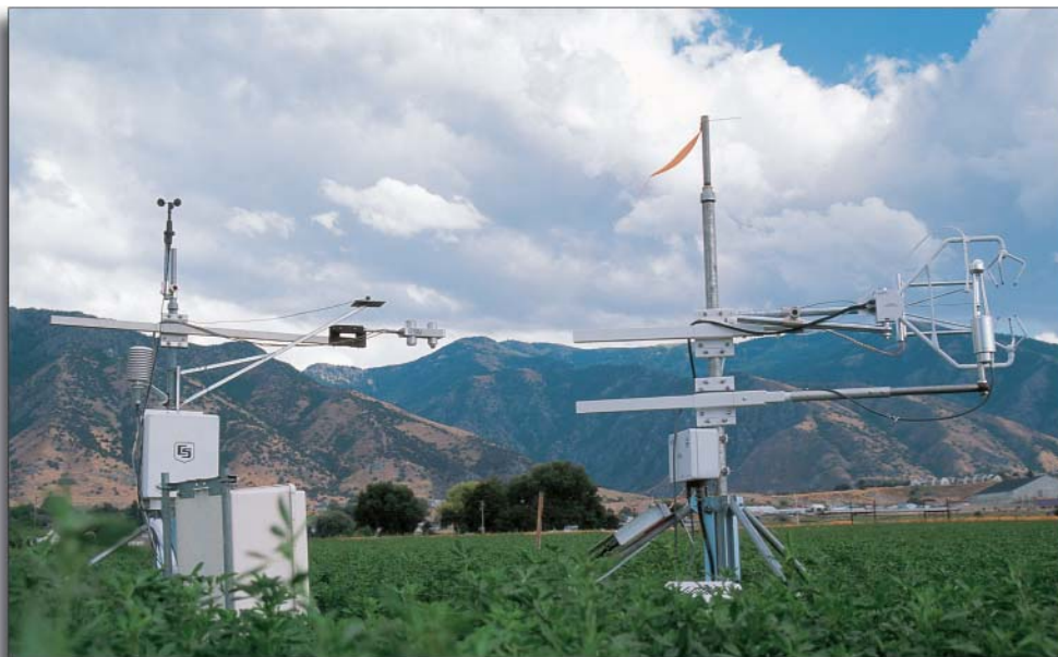
Field intercomparison of fast response sensors measuring surface fluxes of heat, water vapor, and CO 2 (Cache Valley, UT).
