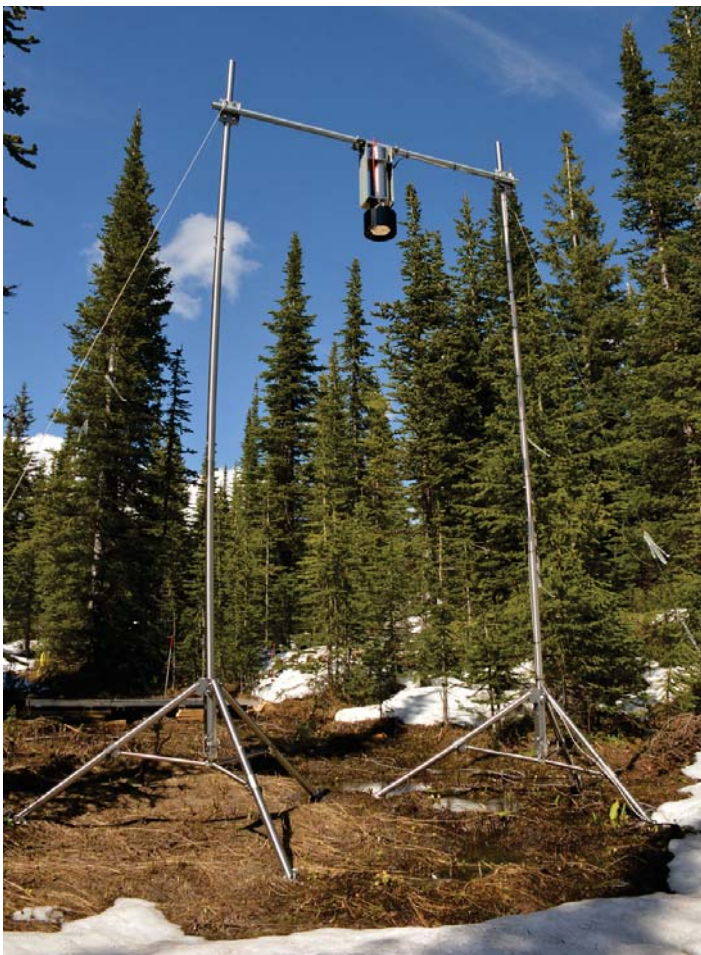
Left & right: The CS725 Snow Water Equivalent Sensor in the field in the rocky mountains near Canmore, AB. Photos courtesy of Centre for Hydrology, University of Saskatchewan. Photographed by Angus Duncan.
