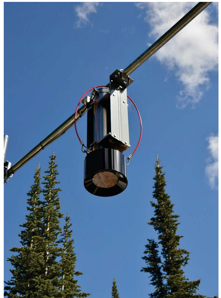
Left & right: The CS725 Snow Water Equivalent Sensor in the field in the rocky mountains near Canmore, AB. Photos courtesy of Centre for Hydrology, University of Saskatchewan. Photographed by Angus Duncan.
