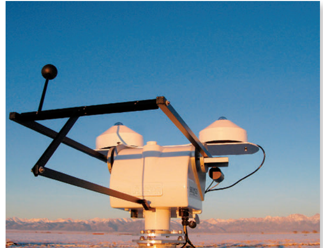
Kipp & Zonen Solys2 Suntracker with Shading Ball Assembly. Measurements of Global and Diffuse radiation are made using the CVF3 ventilation unit and the CMP11 pyranometers.
