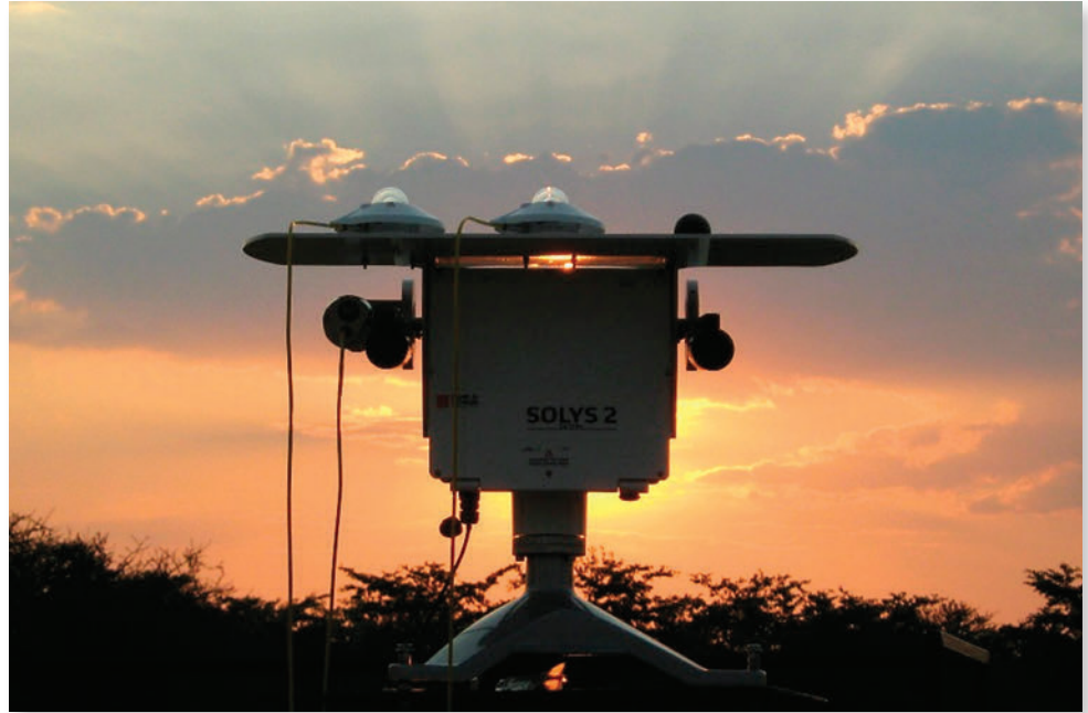
Kipp & Zonen Solys2 Suntracker being used to make measurements of Direct Solar Radiation (CHP1), Global and Diffuse Sky Radiation (CMP11).
