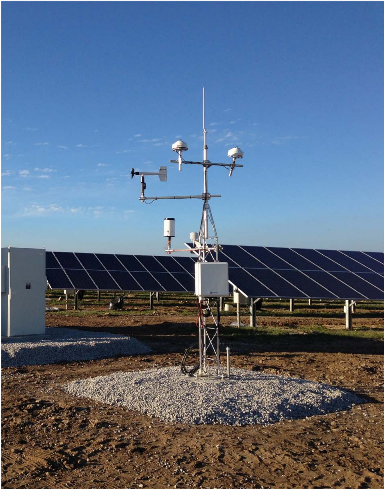
Automated weather station for solar farm performance monitoring. Turnkey systems are available or we can customize your station to meet specific requirements.
