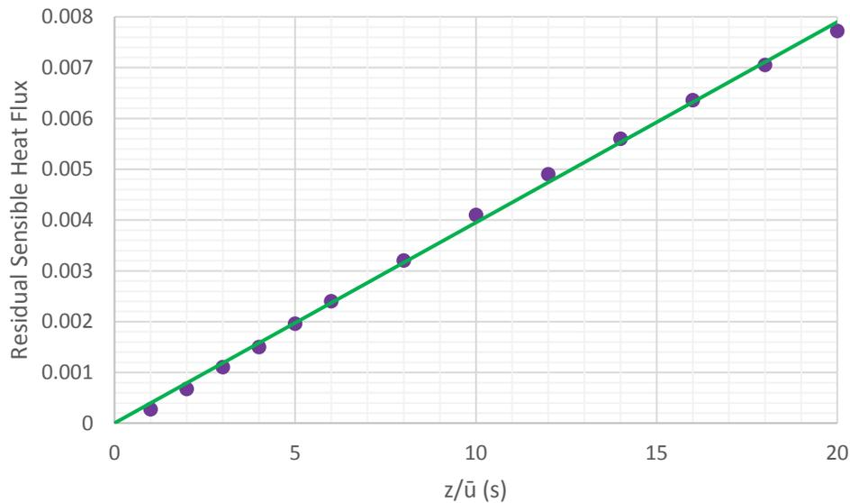
Figure 7. Residual sensible heat flux as a function of  $z/\bar{u}$ .
