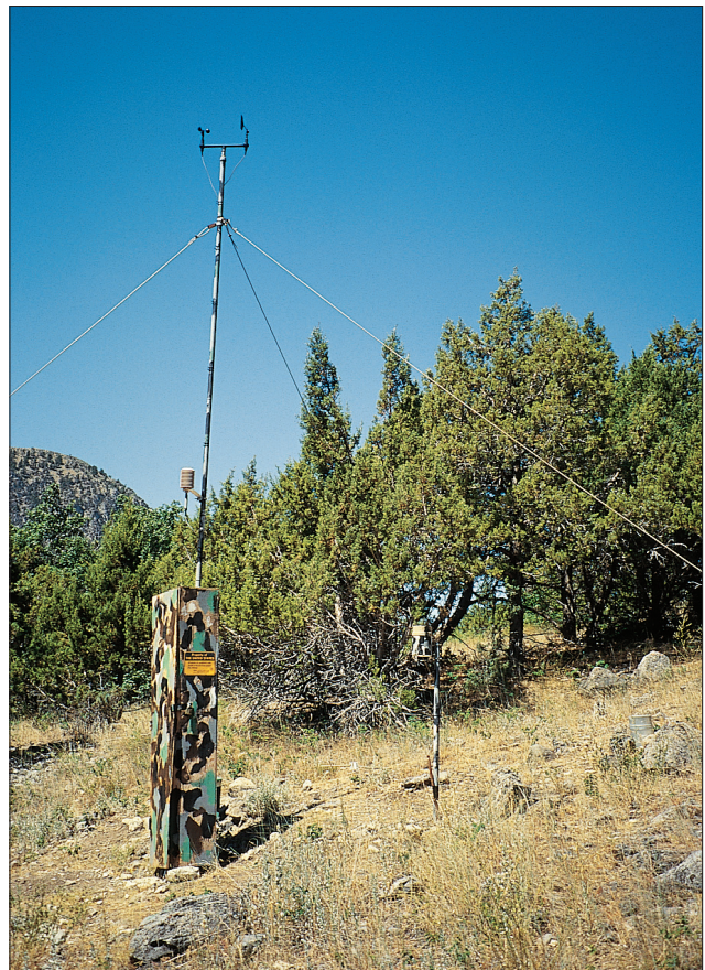
At right is a station that is camouflaged to prevent human pests from damaging it.
