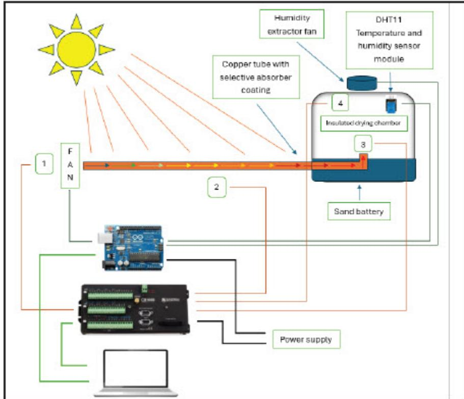
A Campbell Scientific CR1000 Measurement and Control Datalogger, along with T-type thermocouples, monitors temperatures at various points to ensure optimal operation.
