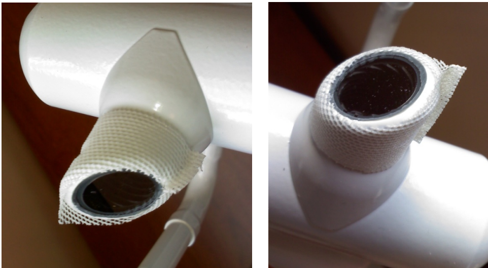
FIGURE 9-3. Proper location of the gas analyzer top wick (left) and bottom wick (right)
