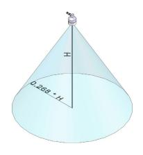
FIGURE 2. Beam Angle Clearance
