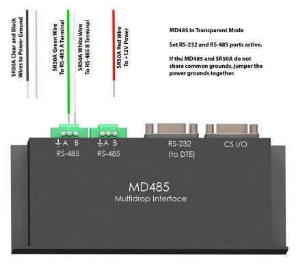
FIGURE 1. SR50A to MD485 Wiring
