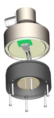
FIGURE 9. Remove Transducer Housing and Disconnect Wires
