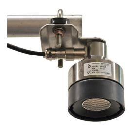
FIGURE 5. The SR50A Mounted to the Crossarm Shown from Another Angle
