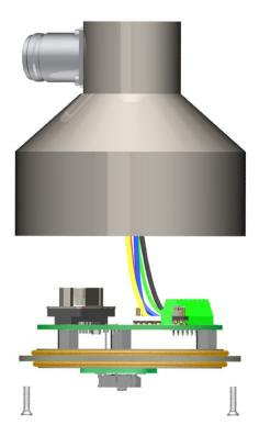
FIGURE 12. Remove the 2 Flat Philips Screws to Expose the PCB
