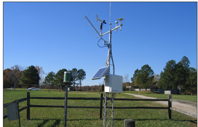
This station for the National Estuarine Research Reserve (NERR) in Virginia transmits data via our GOES satellite transmitter.
