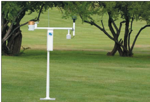
The ET107 is an automated system designed for commercial agriculture, irrigation scheduling, and meteorological applications.
