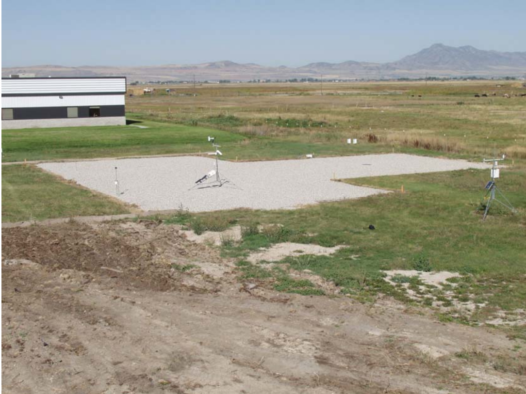
Figure 9. Campbell Scientific, Ltd. Electric Field Meter Site Correction Facility
