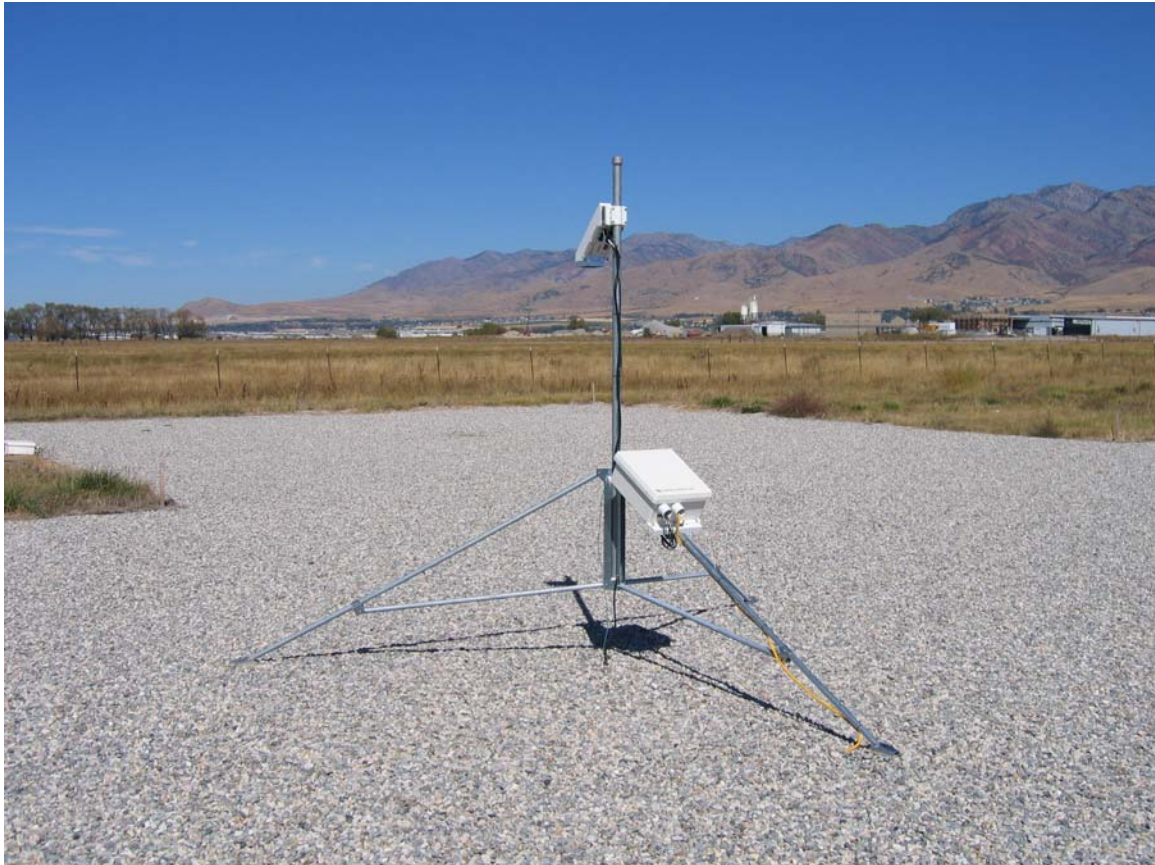
FIGURE G-1. CS110 2 Metre CM10 Tripod Site
