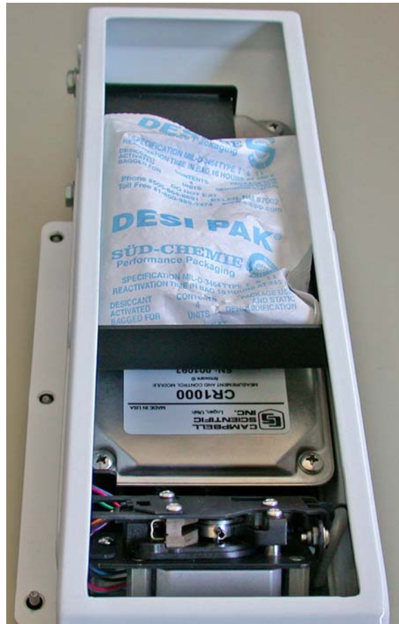
Figure 14. Inside of CS110 Case Illustrating Bracket for Holding Desiccant.
