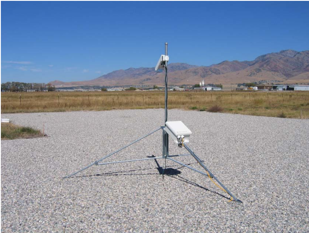
Figure 8. CS110 2 Metre CM10 Tripod Site.
