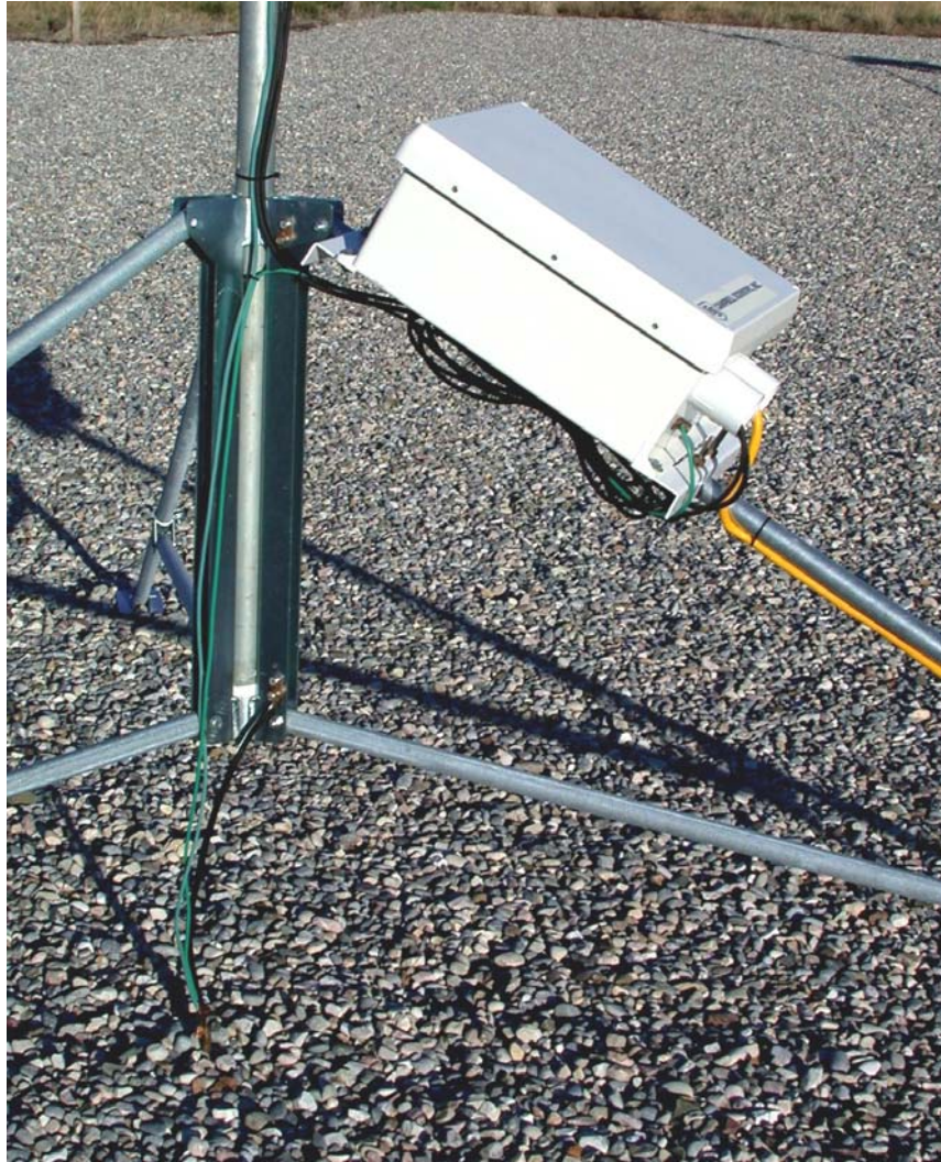
FIGURE G-3. Earth Grounding
