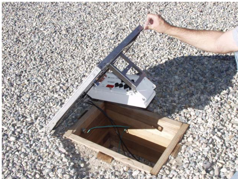
Figure 10. CS110 Attached to Upward-Facing Flush-Mounted Plate for Site Correction
