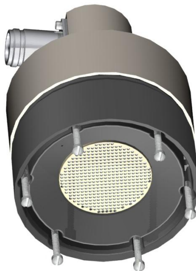
Figure 8. Remove 6 Screws from the Transducer Housing
