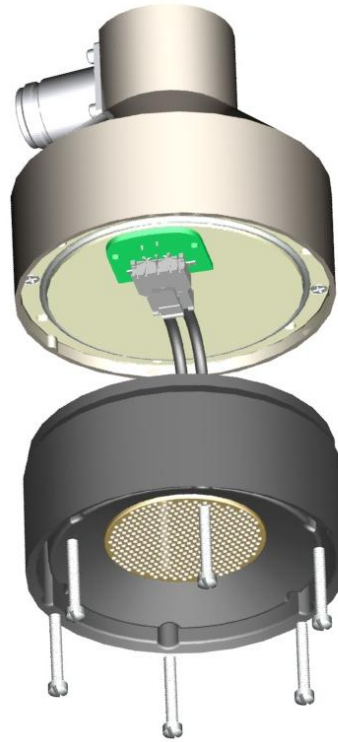
Figure 9. Remove Transducer Housing and Disconnect Wires
