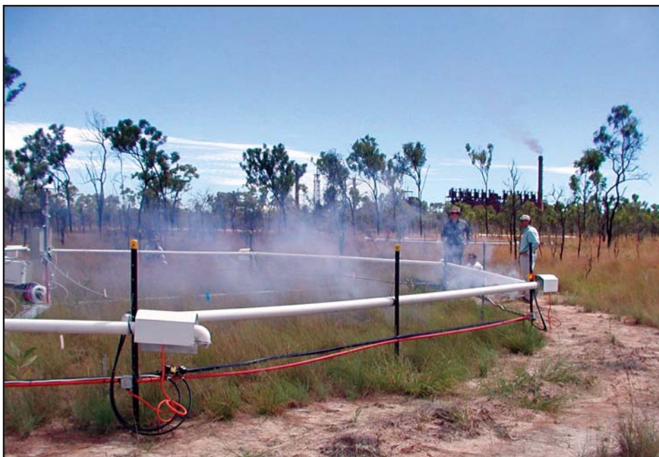
Testing the CO 2 delivery system with a smoke generator during the OzFace installation.
